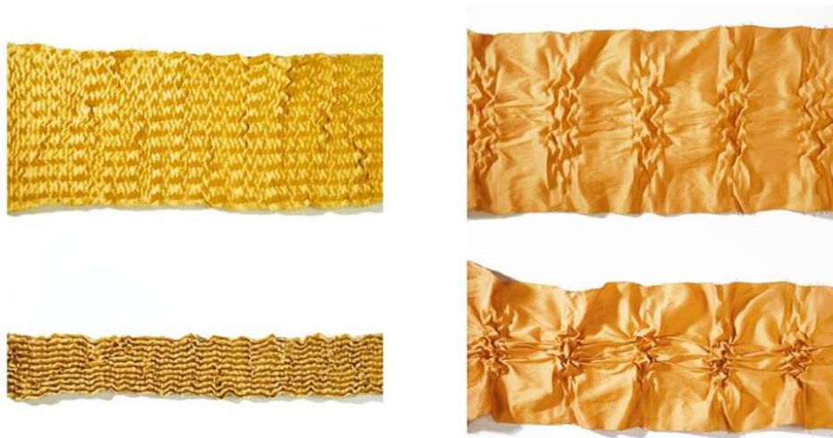
Figure 3 Smart textile employing shape memory wires, Leenders [5]
