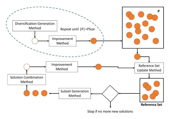
Figure 2: Flowchart of Scatter Search algorithm (Adaptation of Martí and Laguna, 2003).
