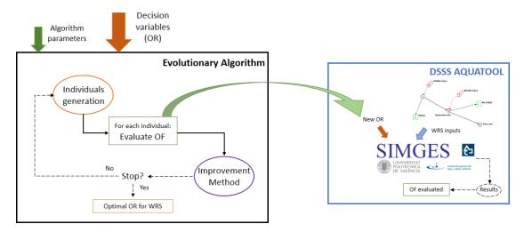
Figure 1: Methodology. EA combined with the network flow SIMGES.
