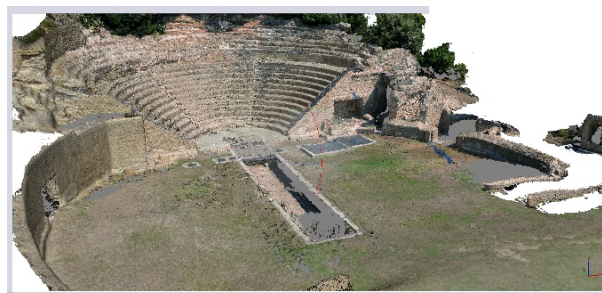
Figure 3: Photogrammetric dense point cloud.
