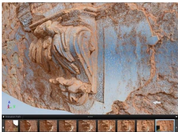
Figure 11: Photogrammetric model of the capitel in mesh view. In the bottom sequence are some of the nine pictures used for its realization.
