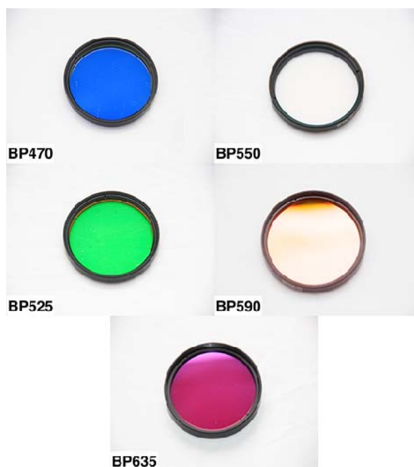
Figure 3: Five bandpass filters used for the testing. The number of MidOpt filter is pointed out in each image.
