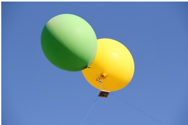
Figure 5: the use of helium balloons to map the valley of Turu Alty.
