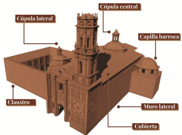
Figure 9: The end result of the reconstruction. They have highlighted the elements of the building that no longer exist today and therefore it has been necessary to go to old photographs in order to figure the hypothesis of reconstruction.
