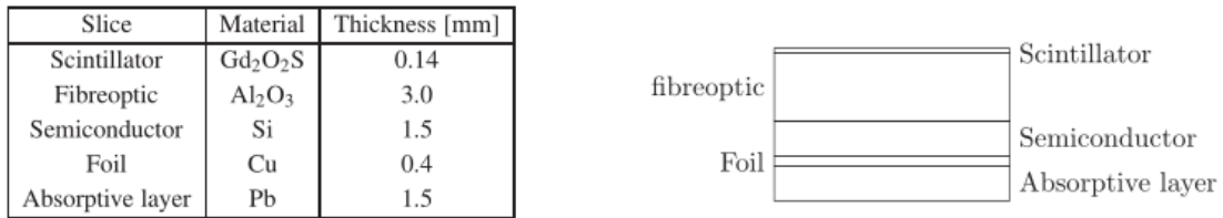
Figure 1. Internal structure of the Hammamatsu C9312SK flat panel, gadolinium oxysulfide (Gd 2 O 2 S) powder phosphor screen.
