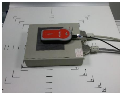
Figure 6. Dose and HVL measures using Piranha detector.
