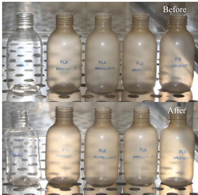
Figure 13. Thermostability test of clay-PLA nanocomposite bottles. Before and after conditioning in the oven of 60 °C. Adapted from [49].
