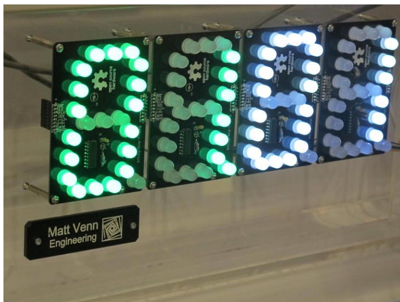
Figure 45 -Array of 4 Big 7 segment displays installed on the final robot.
