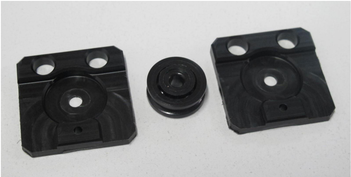
Figure 35 - Delrin enclosure for the pulleys used to redirect the string at the top part of the robot
