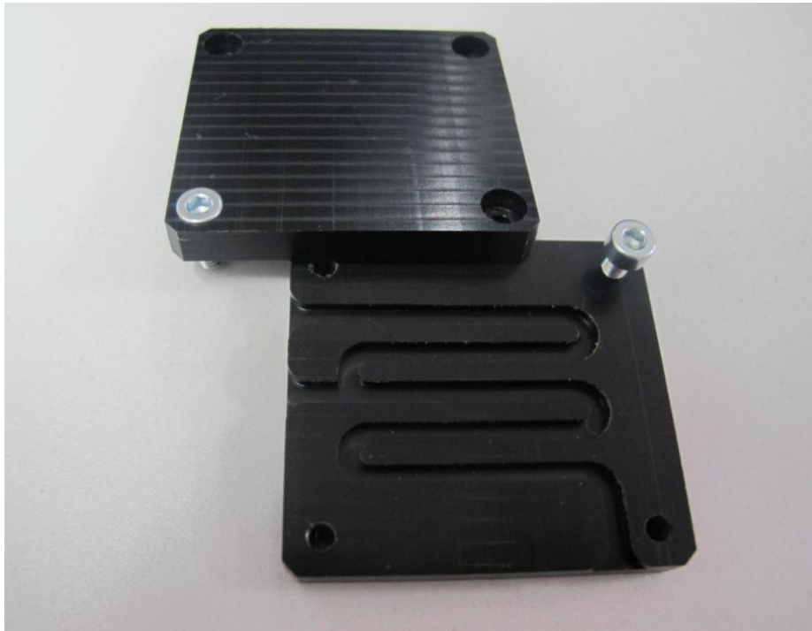
Figure 34 -Delrin tension holder with adjustable friction
