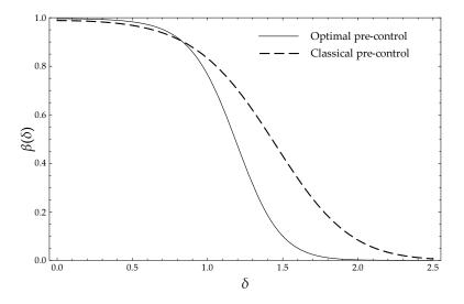
Figure 2: Operating characteristic curves for the classical qualification procedure and the optimal pre-control plan obtained for the example in Section 5.
