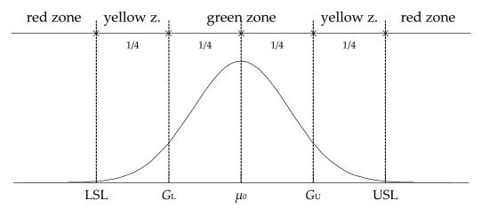
Figure 1: Classification procedure in classical pre-control, for an in-control normal process with potential capability  $C_p = 1$ .
