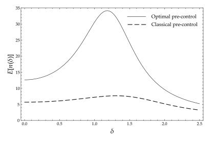
Figure 3: Expected sample size for the classical qualification procedure and the optimal pre-control plan obtained for the example in Section 5.
