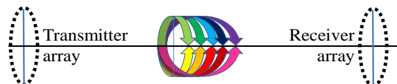
Figure B.3: With circular arrays data streams are mapped onto vortices of various orbital angular momentums.
