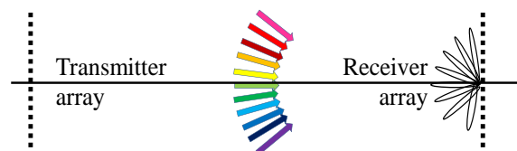
Figure B.2: With linear arrays, data streams are mapped onto angles of arrivals.
