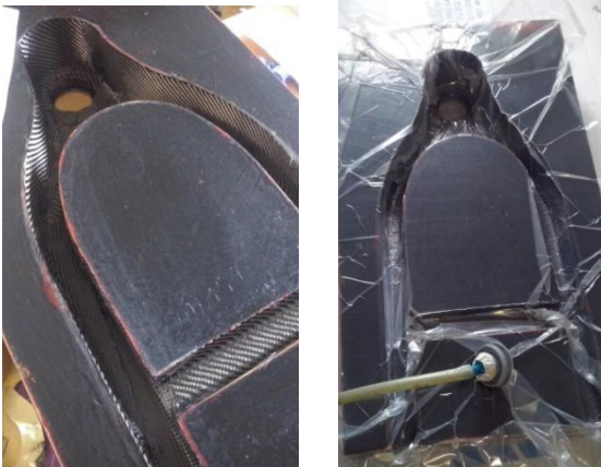
Fig. 13. First layer lamination and compaction in a vacuum bag.
