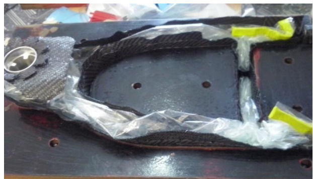
Fig. 17. Vacuum bag positioning. Lateral join flaps detail and joins flaps in the shank.
