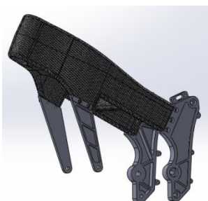
Fig. 2. The final design of the frame in carbon and aluminium.
