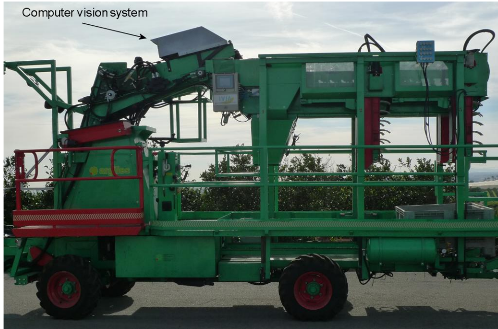
338 339 Figure 8. Mobile platform with the grading system
