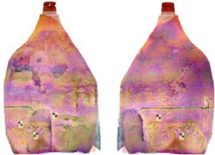
Figure 142. Visible and thermal images overlay of the silo 3.
