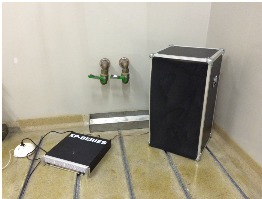
Figure 4 – Speaker used in the Anechoic room for the sound excitation.
