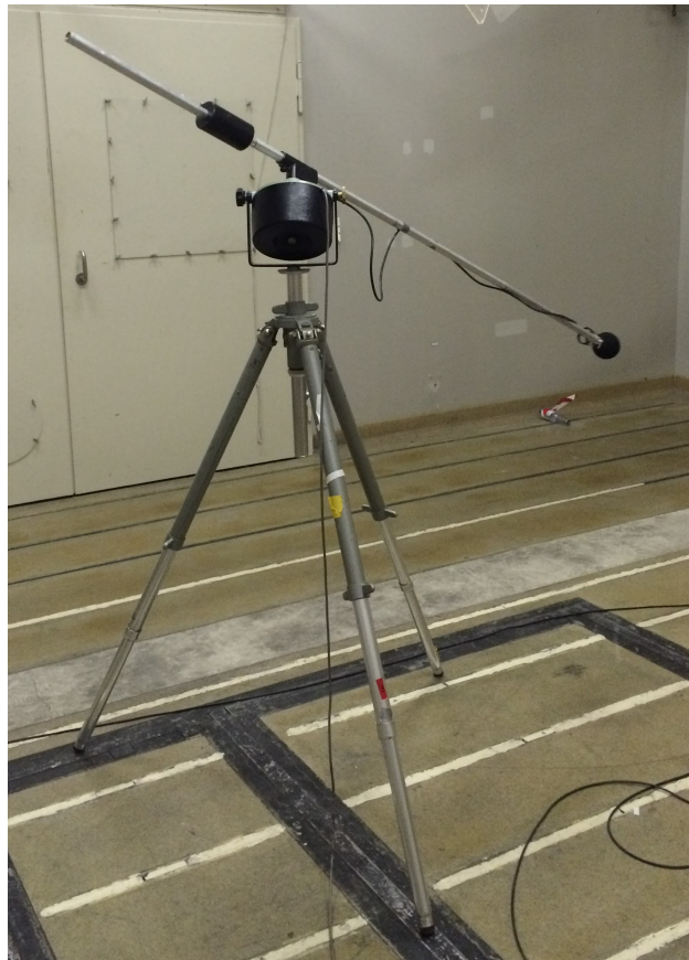
Figure 7 – Microphone boom positioned in the reverberation room.
