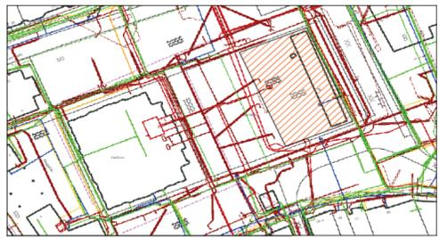
Almost all the pipes and cables are on the left side, so for that reason the design for the new proposals it will take into consideration not to installed fountains and planted trees on the left side, trying to do that on the orange shaded area.
