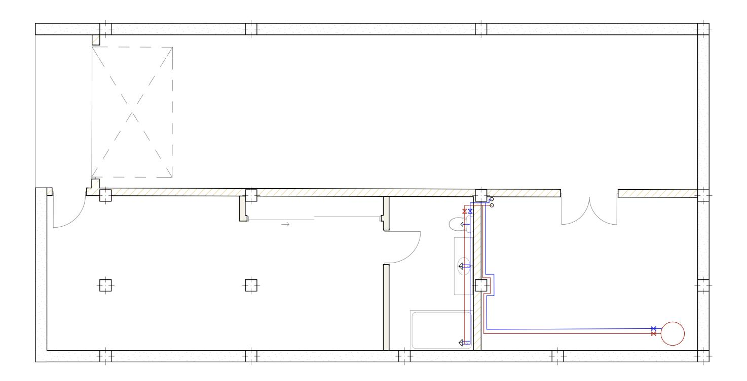
Cold water network Hot water network  $\bowtie$ Individual cut key  $\Rightarrow$ Hidro-mixer  $\rightarrow$ Cold water tap  $\bowtie$ Water meter General key И Pass valve - Stopcock Ο Vertical pipe Heater
