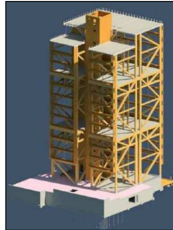
10. Timber structure of the Treet building. – source: ARTEC
