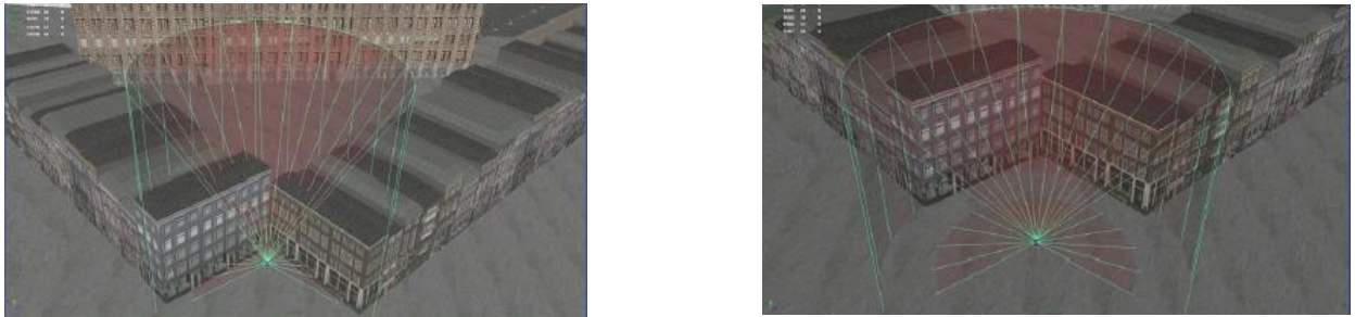
Fig 14 : (left) Bad scanner positioning: presents steep angles. (Right) Good scanner positioning
