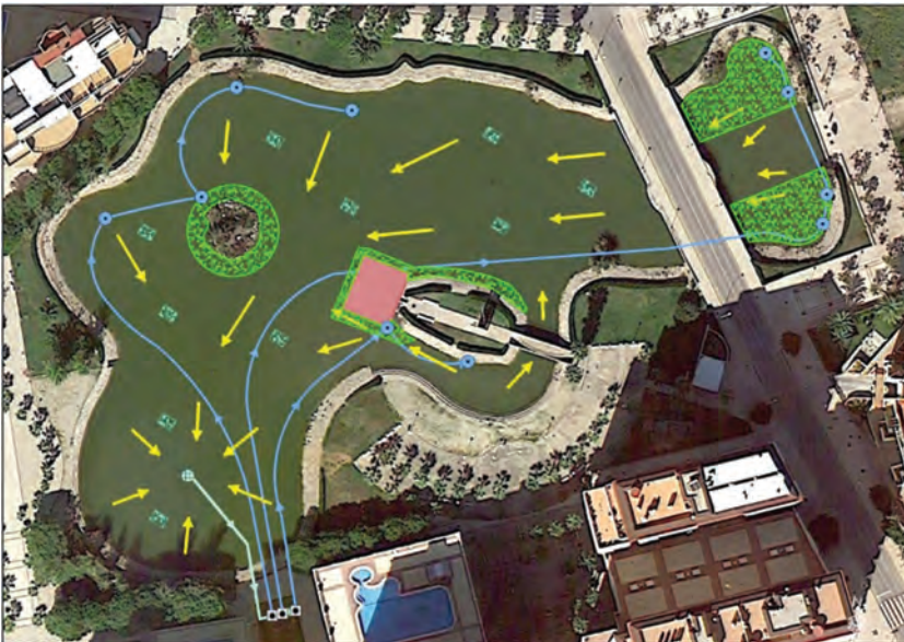
Figure 8: Simulation of biofilters in La Goleta Lake (arrows representing the recirculating water system).
