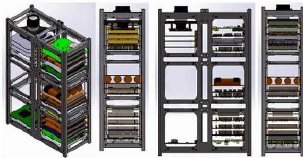
Figure 8.5: Perspective projection of the modules distribution in the 6U structure (Credits: ITA)
