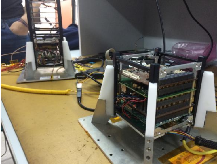
Figure 8.3: Engineering models of a NanosatC-Br1 and NanosatC-Br2
