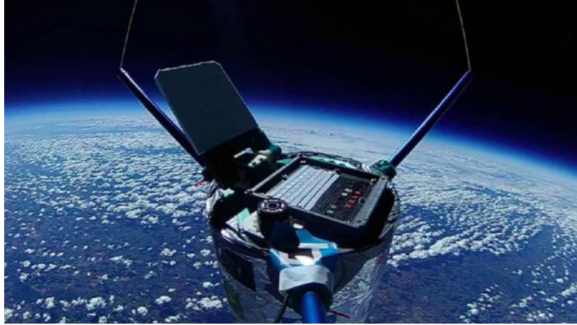
Figure 8.2: Photo taken at the Garatêa gondola in the stratosphere, with bacteria being exposed (All Credits to Zenith)
