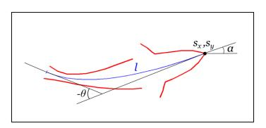
Figure 6: The five parameters  $\boldsymbol{M} = (s_x, s_y, l, \alpha, \theta)$  that define our model.
