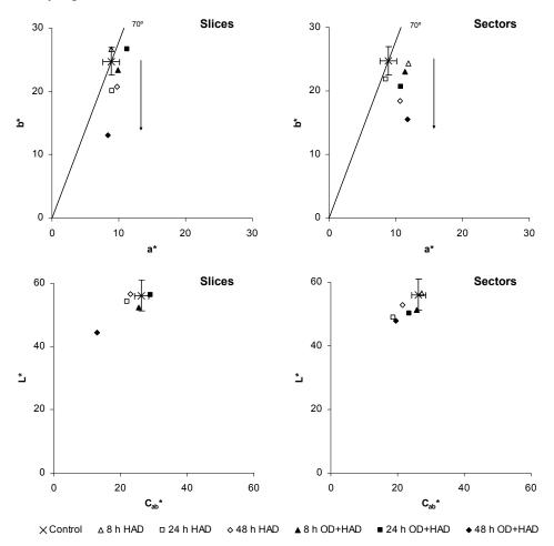
**Figure 3.**  $a^*-b^*$  chromatic diagrams and clarity (L\*)-chrome(C\*<sub>ab</sub>) plains of dried cut persimmon according to drying time and depending on osmotic pre-treatment and shape (0, 8, 24, 48h).
