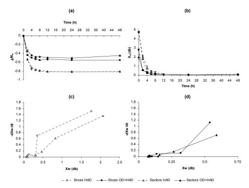
**Figure 1.** Changes of water mass  $(\Delta M_w)$  during the drying stage (a), the drying curve ( $X_w$ : mass ratio of water) (b) and the drying rate curves (c) and (d) of sectors or slices of osmotically pre-treated persimmon (OD+HAD) or not (HAD).
