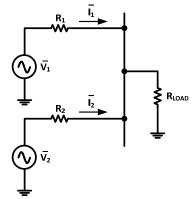
Fig. 4. A pair of generators forming a microgrid
