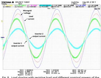
Fig. 9. Load sharing with resistive load and different nominal powers of the inverters (Load 3 kW) (Axis scales: 100V/div; 5A/div)
