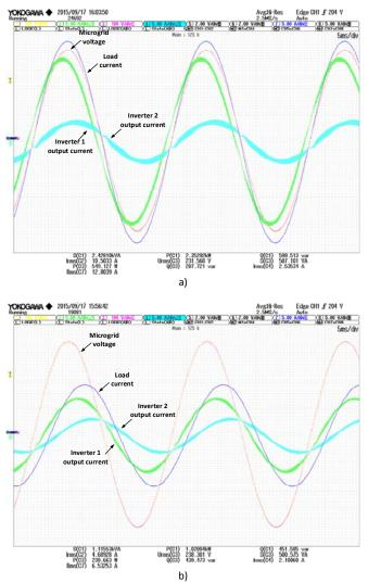
Fig. 11. Load sharing with very different nominal powers of the inverters. A) Resistive load = 3 kW b) RL load = 1.41 kW / PF = 0.71(Axis scales: 100V/div; 5A/div)
