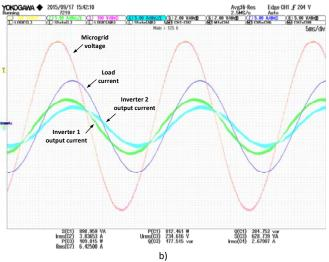
Fig. 10. Load sharing with different nominal powers of the inverters A) Nonlinear load = 1.55kVA, CF = 1.6, DPF = 1 b) RL Load = 1.41kVA / PF = 0.71 (Axis scales: 100V/div; 5A/div)
