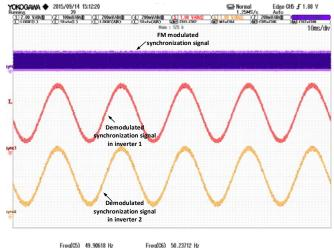
Fig. 5. Demodulated synchronization signals
