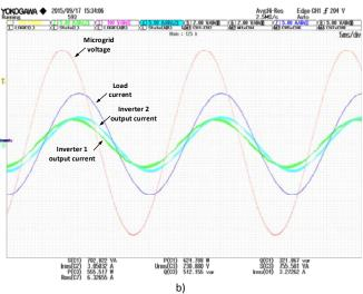
Fig. 7. Load sharing with equal nominal power of the inverters and inductive loads. A) Purely inductive load 1 kVAr b) R-L Load = 1.41kVA / PF = 0.71 (Axis scales: 100V/div; 5A/div)
