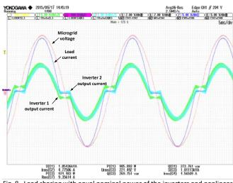
Fig. 8. Load sharing with equal nominal power of the inverters and nonlinear load of 2.4kVA (CF = 1.6, DPF = 1) (Axis scales: 100V/div; 5A/div)
