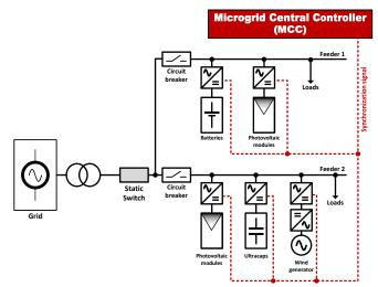
Fig. 1. Microgrid Central Controller (MCC) in an AC microgrid
