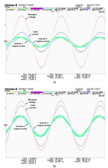
Fig. 6. Load sharing with resistive load and equal nominal power of the inverters. A) Load = 1 kW b Load = 2 kW. (Axis scales: 100V/div; 5A/div)
