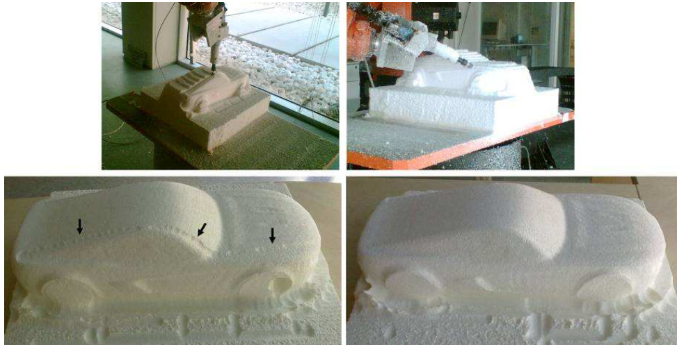
Figure 10. Milling of a small workpiece: bottom left, result without calibration; bottom right, result with calibration.
