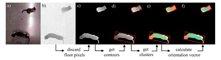
Figure 2. Process of extracting the cat's orientation: (a) color frame (b) depth frame, (c) background segmentation, (d) cat contours, (e) clusters for head, body and tail, (d) orientation vector
