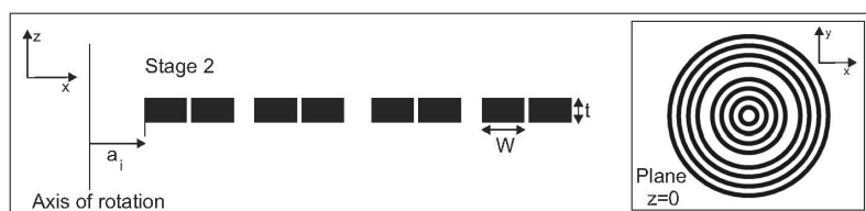
Figure 3. Schematic section diagram of the generation for a FRZP and FRZP considered.
