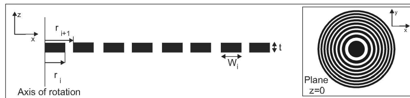
Figure 1. Schematic section diagram of the generation for a Fresnel zone plate (FZP) and FZP considered.
