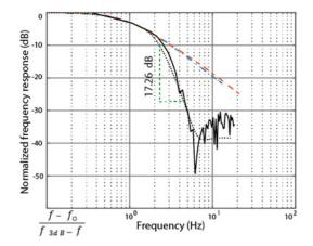
Fig. 5. Bode diagram of the SBS-based filter response. Experimental filter response (black solid) with 16.7 dB/oct; theoretical filter response obtained from (6) (black dotted) with 17.26 dB/oct; theoretical response with a single pump and 5 dB gain (blue dash-dotted) with 3.79 dB/oct; theoretical response with a single pump and 15 dB gain (red dashed) with 4.08 dB/oct.
