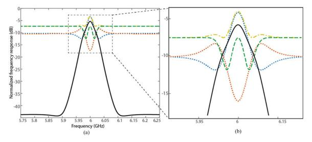
Fig. 2. (a) Evaluation of the terms of (6). (Black solid) Normalized total frequency response of the SBSbased filter obtained from (6). (Blue dotted) Amplitude frequency response of the gain SBS response (lower sideband), i.e. first term of (6). (Red dotted) Amplitude frequency response of the loss SBS response (upper sideband), i.e., second term of (6). (Yellow dot-dashed) Combination of the first and second terms of (6). (Green dashed) third and fourth term of (6). (b) Detail of Fig. 2(a).
