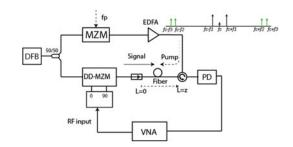
Fig. 3. Block diagram of the experimental setup. DFB: distributed feedback laser, MZM: Mach-Zehnder modulator, DD-MZM: Dual-Drive MZM, VNA: vector network analyzer.
