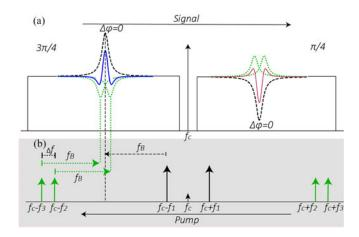
Fig. 1. Principle of operation. (a) Optical spectrum of the forward signal with SBS amplitude gain and loss responses. (b) Backward pump signals with frequency  $f_p$ , where p = 1, 2, 3.
