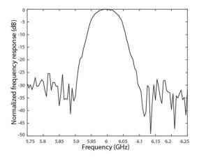
Fig. 6. Normalized RF frequency response of the SBS-based filter with 84 MHz FWHM bandwidth.
