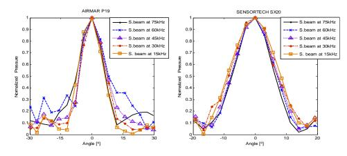
Fig. 3. Beamwidth measured at different parametric frequencies for AIRMAR P19 transducer (left), and Sensortech SX20 (right).
