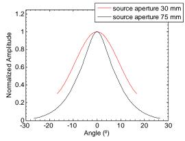
Fig. 5. Parametric beamwidth comparison between a source aperture of 30mm of diameter against 75mm one
