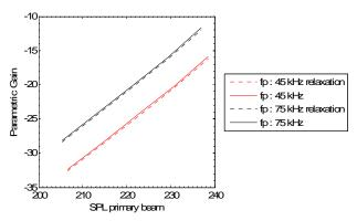
Fig. 4. Parametric gain for two frequencies (45 kHz and 75 kHz). Comparison between the numerical model without relaxation losses and with them.
