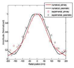
Fig. 2. Primary and secondary beamwidth comparison for numerical and experimental result for a parametric frequency of 45 kHz.
