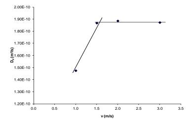
Figure 9. Influence of air velocity on drying kinetics at 70°C (no ultrasound application)
