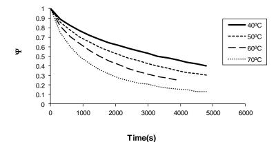
**Figure 2.** Experimental drying kinetics at different temperatures and an air velocity of 1 m/s (without ultrasound application)
