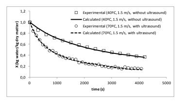
**Figure 5.** Comparison between modeled by Peleg's model and experimental drying curves for two drying conditions (40°C, 1.5 m/s, without ultrasound and 70°C, 1.5 m/s, with ultrasound)
