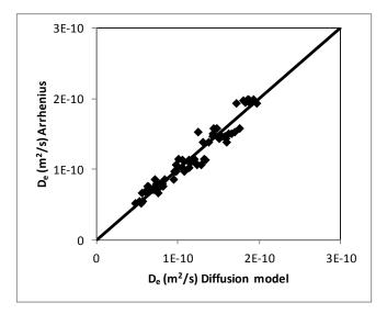
**Figure 8**. Values of  $D_e$  calculated by Arrhenius equation versus  $D_e$  from diffusion model for all the temperatures under study
