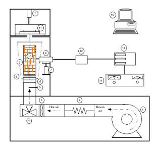
**Figure 1.** Convective dryer. (1) Fan; (2) Heating; (3) Anemometer; (4) Pneumatic three-way valve; (5) Temperature probe Pt-100; (6) Coupling material; (7) Elevator; (8) Ultrasonic transducer; (9) Braces; (10) Parallel plate support; (11) Scale; (12) Impedance matching unit; (13) Digital watimeter; (14) Generator of power ultrasound; (15) Computer-controller.
