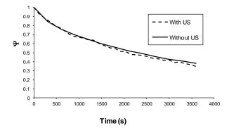
Figure 4. Experimental drying kinetics at 40 °C and 1m/s with and without ultrasound application
