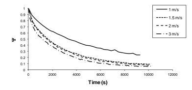
**Figure 3.** Experimental drying kinetics at different air velocities and a temperature of 40°C (without ultrasound application)
