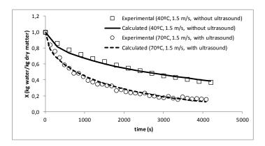
**Figure 6**. Comparison between modeled by diffusion model and experimental drying curves for two drying conditions (40°C, 1.5 m/s, without ultrasound and 70°C, 1.5 m/s, with ultrasound)
