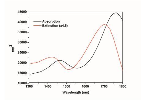
Figure 6. Nanostrip's scattering spectra illuminated with a plane wave and surrounded by an effective refractive index  $n_{eff}$ =2.32. The dimensions of the coupled systems are as in the asymmetric configuration of Fig. 2.
