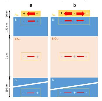
Figure 5. Schematic representation of the image currents in a system consisting of a plasmonic nanostrip (supporting a dipolar (a) or a quadrupolar (b) electric resonance) on top of a siliconon-insulator wafer (dimensions not to scale). Accumulation of charges is represented by '+' or 'signs whilst the arrows stand for the currents (and the thickness of the arrows stand for the current strength).
