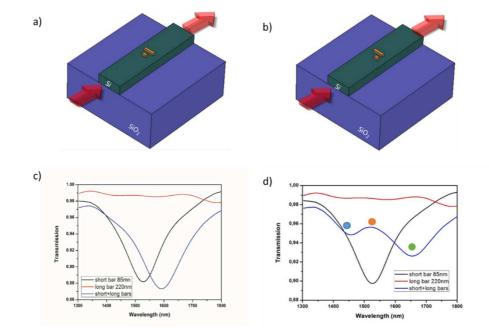
Figure 2. Schematic with the two coupled nanostrips on the silicon waveguide with (a) symmetric and (b) asymmetric -  $\Delta x_1 \neq 0$  for the short nanostrip - configuration. The blue curve represents the transmission for the (c) symmetric configuration showing no Fano effects and for the (d) asymmetric configuration showing Fano effects. Also, in black (red) the case when only the short (long) nanostrip is considered on top of the silicon waveguide.
