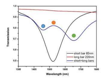
Figure 7. Transmission for the asymmetric configuration showing Fano and EIT behavior for a chain of five resonators separated 155nm. The extinction ratio is greatly enhance whilst the Fano asymmetric profile is maintained.
