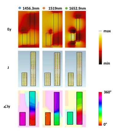
Figure 4. Electric field's parallel component to the nanostrips (top), surface current distribution (middle) and phase of the surface current distribution parallel component to the nanostrips (down) computed at three different wavelengths in the Fano resonance (see Fig. 2d).
