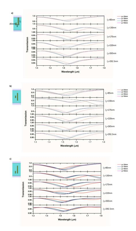
Figure 3. Variation of the transmission with the long nanostrip length l₂ and its separation g to the short nanostrip, with the short (a), both (b), or the long (c) nanostrips centered in the middle of the waveguide as depicted in the sketch of each figure. Notice that the right selection of the physical dimensions of the coupled system can give rise to the pursued Fano response.
