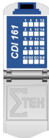
Figure 2.12: Module CDI-161 Status display
