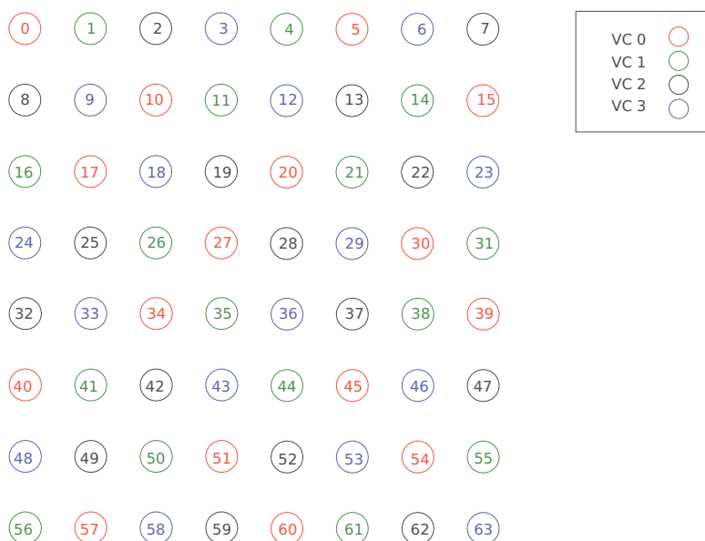
FIGURE 11.4: How XORDET assigns destinations to VCs in a 8 \times 8 mesh with 4 VCs.
