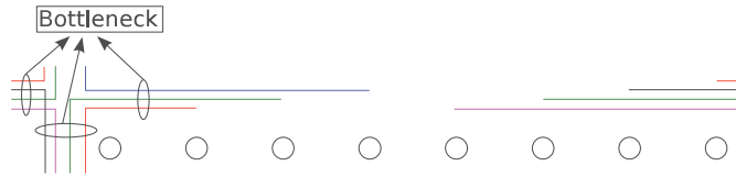
FIGURE 10.1: Paths of source-destination pairs of the first row with Bit-reversal pattern traffic.
