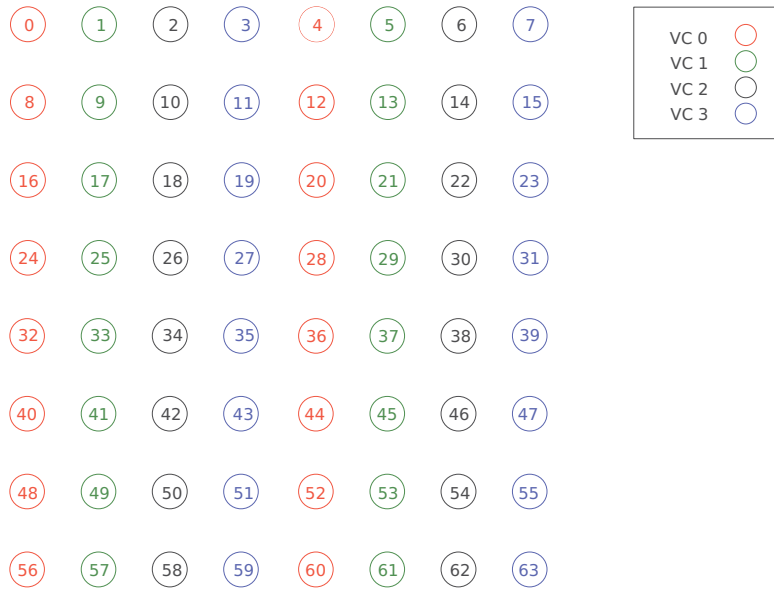
FIGURE 11.1: How DBBM assigns destinations to VCs in a 8 \times 8 mesh with 4 VCs.
