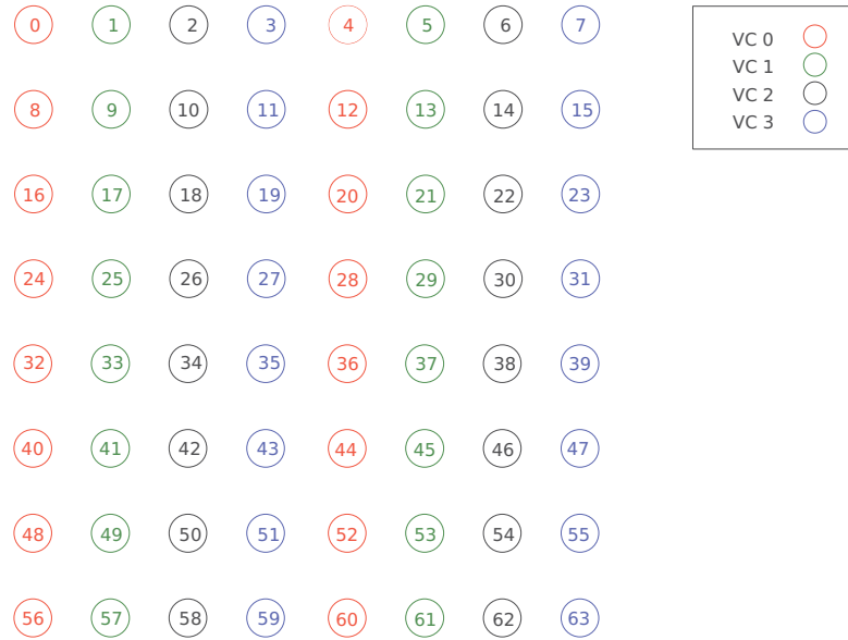
FIGURE 1.2: How DBBM assigns destinations to VCs in a 8 \times 8 mesh with 4 VCs.
