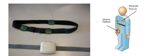
**Figure 7**. Illustration of R-TIPS. This platform allows monitoring of the cardiac signal wirelessly. It is composed by transmitter system and three sensors (see a). The transmitter system are placed in the participant's hip and the sensors are placed, one in the below right breast, other in the right side and the last in the back (see b).
