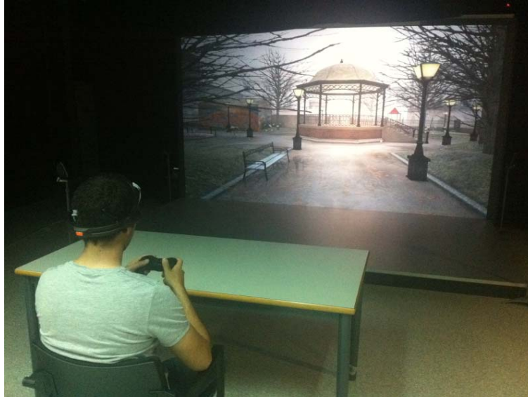
Figure 2. Subject navigating in the virtual environment while brain activity is monitored with Emotiv EPOC
