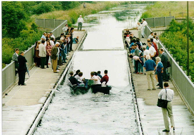
Figure 2.16: Soliton on the Scott Russell Aqueduct on the Union Canal near Heriot-Watt University, 12 July 1995. Photo from Nature v. 376, 3 Aug 1995.
