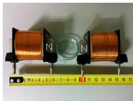
Figure 5. Experimental setup. Water or PVA solution was placed in a Petri dish between two electromagnets. The magnetic flux density in the gap depends on the current intensity.
