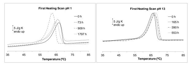
Figure 6. Endothermic DSC curves for the first scan in acid medium, pH 1 (left) and basic medium pH 13 (right)
