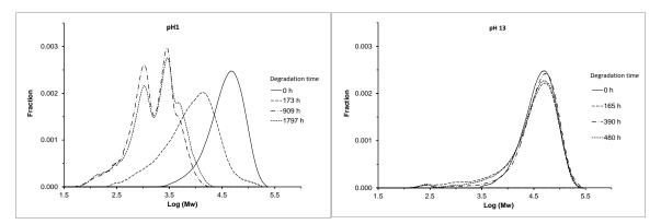
Figure 5 . Molecular weight distribution vs. time degradation in acid medium pH 1(left) and in basic medium pH 13 (right).
