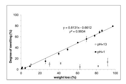
Figure 2. Degree of swelling as a function of weight loss. Straight line represents the linear fit of data corresponding to pH 1.
