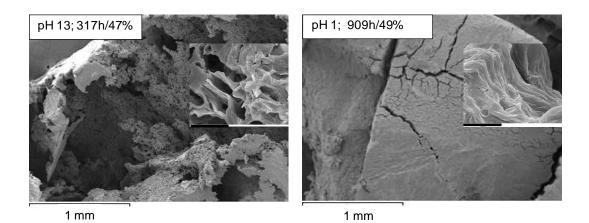
Figure 4. Superficial SEM microphotograps of samples at different degradation times for samples degraded at pH 13 after 317 h and 47% of weight loss (left) and at pH 1 after 909 h and 49% of weight loss (right). The insets show a higher magnification (bar=10µm)
