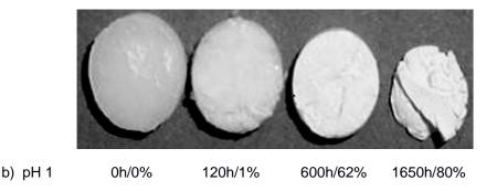
Figure 3- Photographs of samples at different degradation time for samples immersed in a) basic pH 13 and b) acid pH 1 media. Labels indicate degradation time in hours and percentage weight loss.
