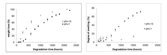
Figure 1. Weight loss profile (left) and degree of swelling (right) as a function of degradation time. Error bars represent standard deviation.
