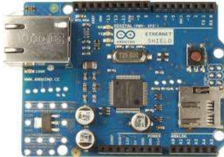
*Figura 4. Shield Ethernet*
