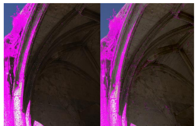
Figure 6: The LDR has almost no keypoints in the shade. However, in the Mantiuk's toned-mapped image the distribution of the detected keypoints is more uniform as the detector finds keypoints even in the darkest area. Image from Château des Baux case study.
