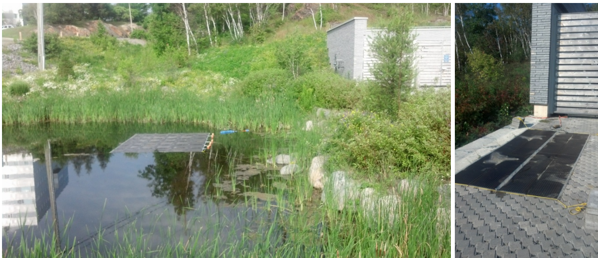
Figure 3: MIRARCO's Floating PV Prototype (Left) and the control ground mounted nearby panels (Right) – Sudbury, Canada
