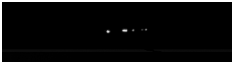
Figure 14 – Example of Multipoint Plasma Induction registered for the condition of 63bar and 700K at 6mm from the injector Nozzle.
