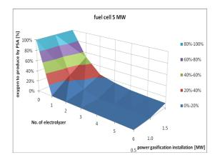
**Figure 8:** Percentage of oxygen produced by the PSA system from the air that gasifier need, for different biomass upgrade gasifier power and number of electrolysers, with 5 MW fuel cell set power. Scenario number 1: 12/12.
