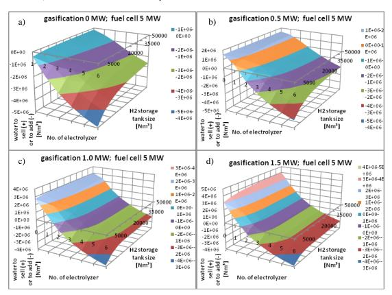
**Figure 6:** Excess of hydrogen production for different biomass upgrade gasifier power: a) 0 MW, b) 0.5 MW, c) 1 MW and d) 1.5 MW, with 5 MW fuel cell set power. Scenario number 1: 12/12.
