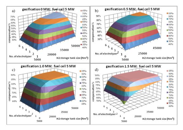
**Figure 4:** Compensation factor of the system for different biomass upgrade gasifier power: a) 0 MW, b) 0.5 MW, c) 1 MW and d) 1.5 MW, with 5 MW fuel cell set power. Scenario number 1: 12/12.
