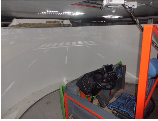
Figure 5. Driving simulation cabin with projection system composed by 3 projectors and a semicircular screen.
