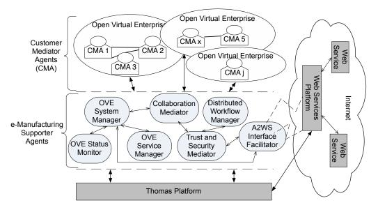
Figure 10: System Architecture of ASeM
