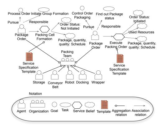
Figure 5: Agent Model of a Package Order Agent of a Packing Cell System
