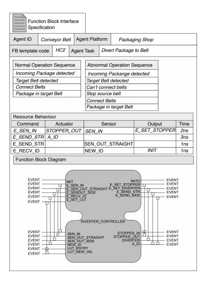
Figure 6: Function Block Specification Interface of the Conveyor Belt Agent of a Packing Cell System
