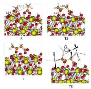
**Figure 5.** PW91 optimized geometries of reactant (R), transition state (TS) and  $\beta$ -keto acid intermediate (I) involved in the C–C bond forming step of acetic acid decarboxylation, and
