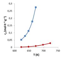
**Figure 2.** Initial reaction rates  $r_0$  (in mol h<sup>-1</sup> g<sup>-1</sup>) for the ketonic decarboxylation of pentanoic (blue  $\blacksquare$ ) and 2-methylbutanoic (red  $\blacklozenge$ ) acids over m-ZrO<sub>2</sub> at different reaction temperatures. Reaction conditions: W = variable, mass flow rate = 36.0 g h<sup>-1</sup>
