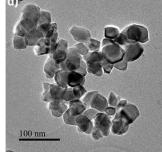
Figure 6. TEM micrographs of  $ZrO_2$  samples a) as purchased and calcined at b) 923 K, c) 1023 K and d) 1123 K.
