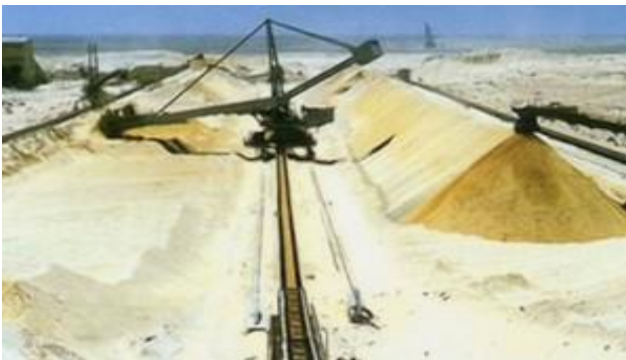
Phosphate bucraa and conveyor tape, Source: Libertad digital
