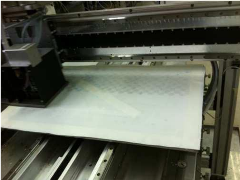
Figure 3: Digital Functionalization. Experiment printing a checked pattern with finishing agent
