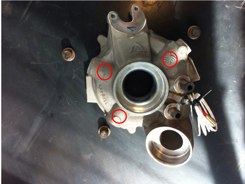
Figure 3.10: Location of the drills for thermocouples installation in LPC volute
