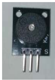
Fig. 8. Buzzer module placed near to the driver's ear.
