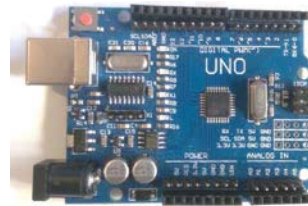
Fig. 3. Processing Unit used in the design of our Low-cost vehicle driver assistance system
