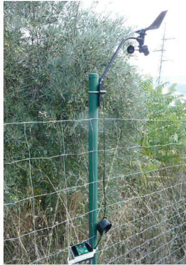
FIGURE 5: Image of a sensor node located at the boundaries of an area of interest, including an anemometer.
