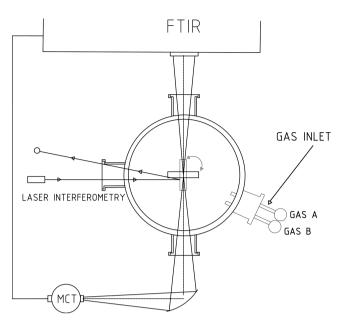
Figure 1. Scheme of the experimental setup for IR spectroscopy measurements.
