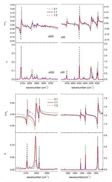
Figure 7. Optical constants in the more relevant NIR and MIR spectral regions of  $CH_4$ :  $C_2H_4$  ices with proportions (3:1), (1:1) and (1:3) at 30 K. Files with the optical constants determined in this work for pure species and mixtures are given in the supplementary material.
