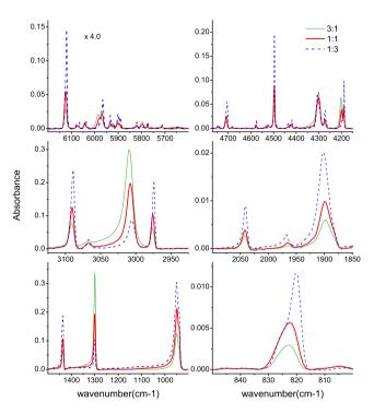
**Figure 5.** IR spectra of CH<sub>4</sub>: C<sub>2</sub>H<sub>4</sub> ice mixtures at 30 K with different composition ratio (3:1, green, thin line, 1:1, red, thick line, and 1:3 blue, dashed line). Ice thickness is 6.5  $\mu$ m in top panels (NIR) and 1.4  $\mu$ m in the others (MIR). Files of the spectra presented in the figure are given in the supplementary material.
