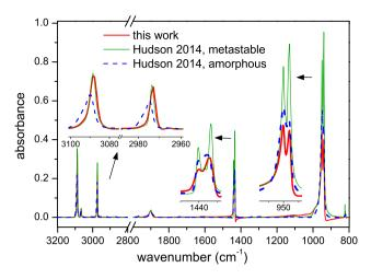
**Figure 3.** Comparison of IR pure ethylene spectrum obtained in this work with previous literature spectra by Hudson et al. (2014), all at 30 K. The literature spectra correspond to ices 0.931  $\mu$ m thick (metastable) and 2.85  $\mu$ m thick (amorphous) and have been multiplied by 1.5 and 0.49 to compare with the 1.4- $\mu$ m-thick spectrum obtained in this work.
