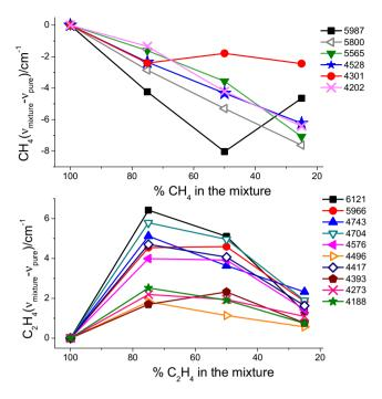
**Figure 6.** Methane (upper panel) and ethylene (bottom panel) band shifts for several NIR absorptions in binary mixtures. The band centres (in cm<sup>-1</sup>) for the various bands of CH<sub>4</sub> and C<sub>2</sub>H<sub>4</sub> are listed in the upper and lower panels, respectively. Files with all the band shifts measured in this work are provided in the supplementary material.
