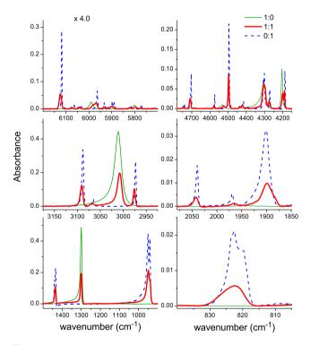
**Figure 4.** IR spectra of pure CH<sub>4</sub> (1:0, green, thin line), pure C<sub>2</sub>H<sub>4</sub> (0:1, blue, dashed line) and a 50 per cent number molecule mixture (red, thick line) ices deposited at 30 K. Ice thickness is 6.5  $\mu$ m in the top panels (NIR) and 1.4  $\mu$ m in the others (MIR). Files of the spectra presented in the figure are given in the supplementary material.
