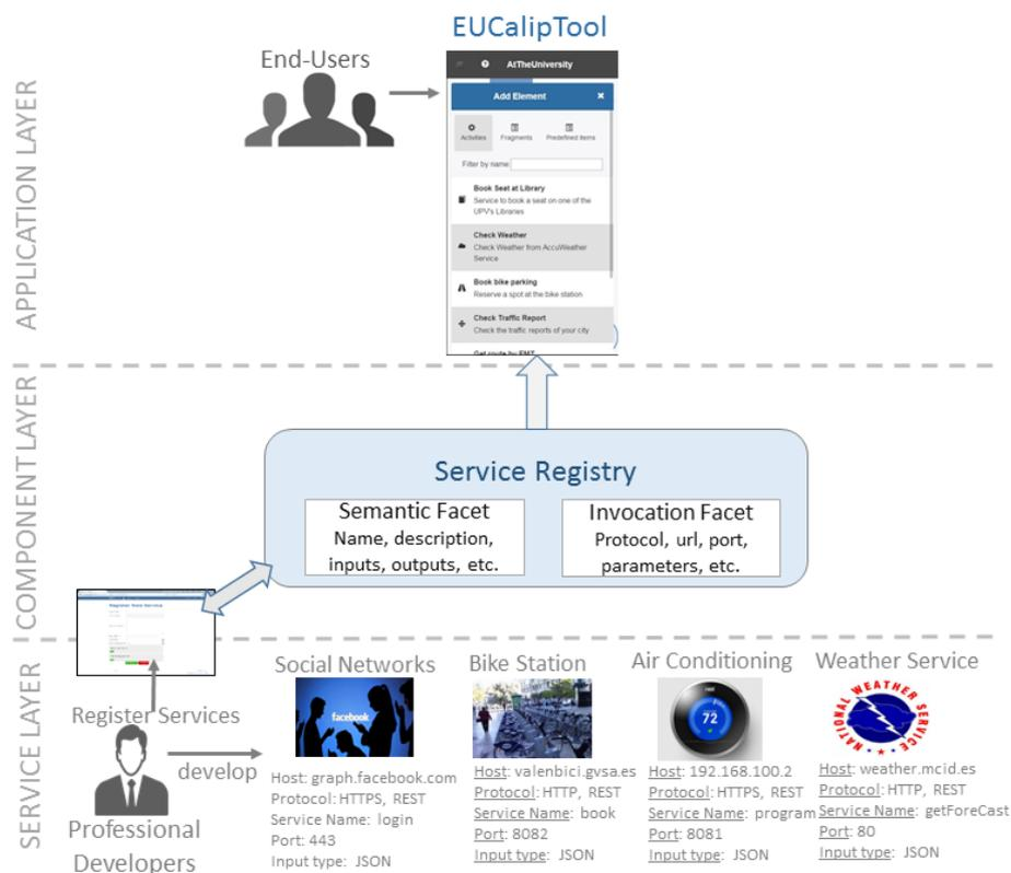
Figure 17. Software Architecture
